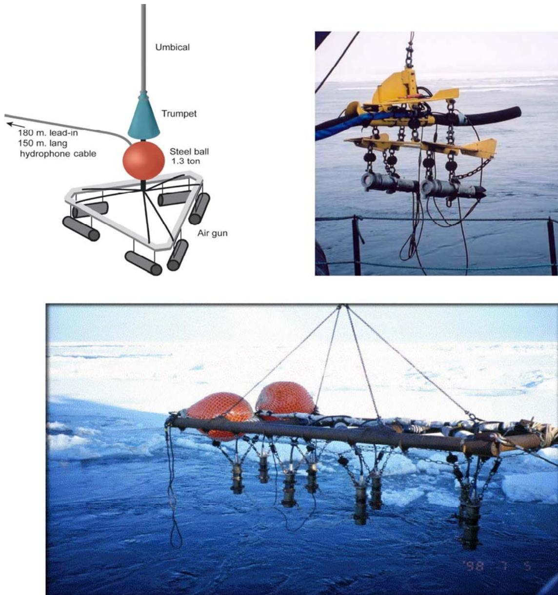
*Fig. 5.2 Seismic source configurations used for seismic reflection measurements in the Arctic Ocean. Upper left: system used in single ship operation by Grantz et al. (1993); upper right; by Kristoffersen et al. (2001), and lower panel: air gun array used by Jokat et al. (1999) in a nuclear icebreaker assisted operation.*
