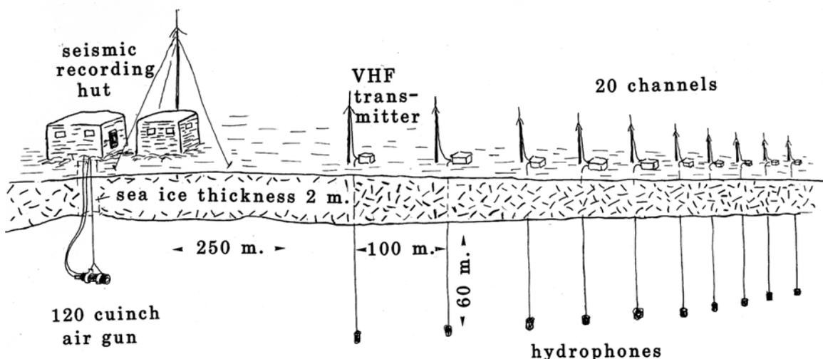
Fig. 5.1 Array of modified sonobuoys used for seismic multi-channel seismic reflection measurements on drifting sea ice. From Kristoffersen and Husebye (1985).
