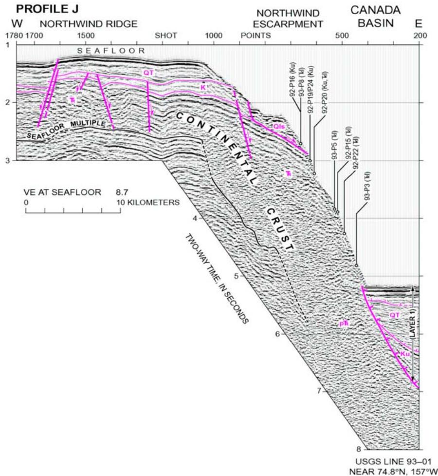
Fig. 6.1 . Seismic reflection profile 93-01 showing the structure and inferred stratigraphy and location of piston cores that sampled bedrock on the adjacent part of Northwind Escarpment. *Qls*-submarine slide; *QT*-Quaternary and Tertiary; *K*-Cretaceous; *Tr*-Triassic; *pTr*-pre-Triassic. (Figure courtesy of A. Grantz)
