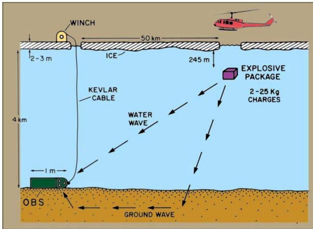
Fig. 4.10 Cartoon showing the procedure for seismic refraction experiment used by Jackson et al. (1982)
