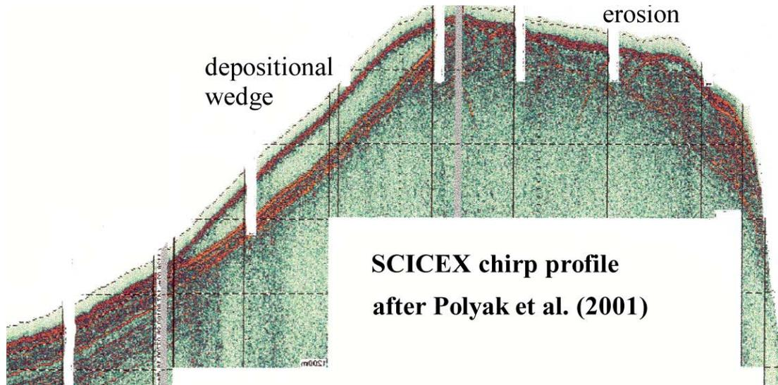
*Fig. 5.3 Example of SCICEX chirp sonar profile across Lomonosov Ridge. Depth scale is 50 m between dashed horizontal lines. After Polyak et al. (2001).*
