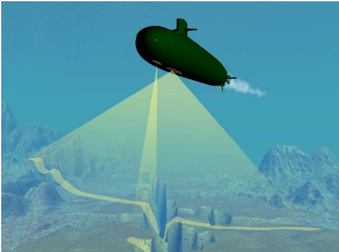
*Fig. 4.7 The concept for seabed mapping and characterization from a nuclear submarine platform as successfully carried out by U.S.N. Hawkbill in 1999 (Figure courtesy of Paul Bienhof).*
